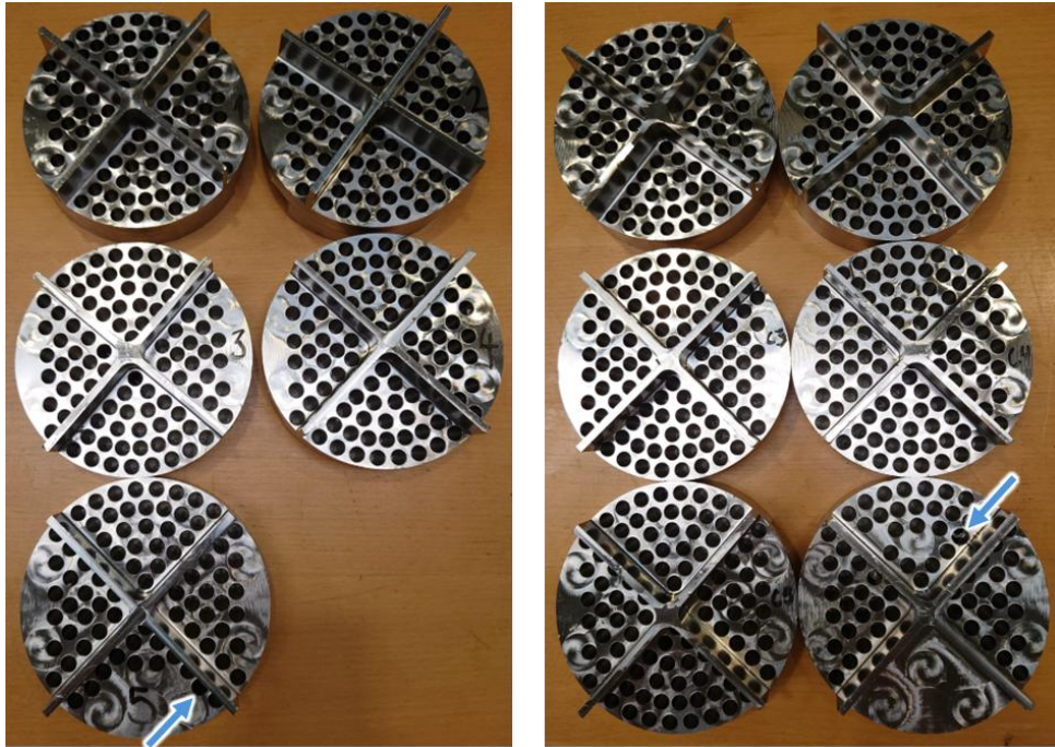
Figure 18 - Drilling comparison, on the right, the untreated tool, on the left, the cryo-treated tool results. In each case, a blue arrow is pointing to the hole where the tool broke.
