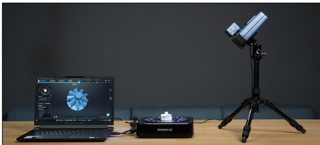
Figure 10 - Turntable Scanning (Einscan, 2018)
