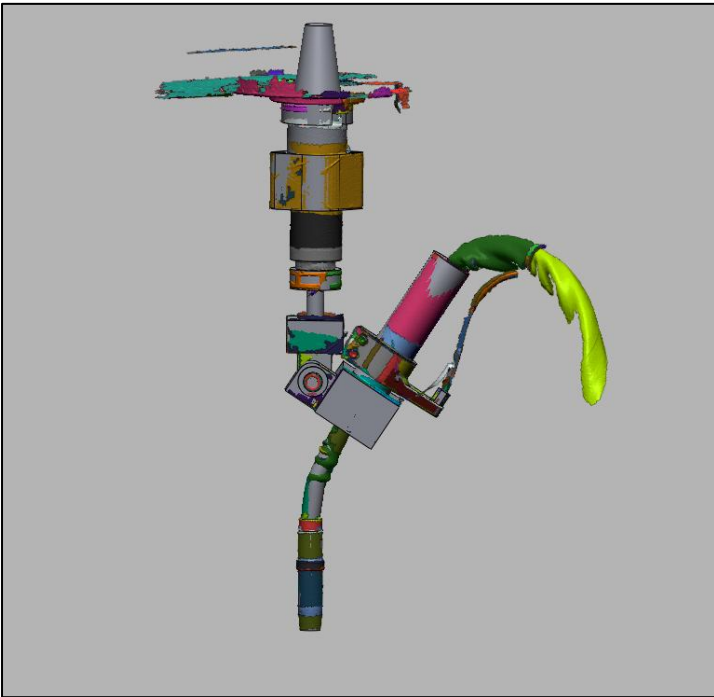
Figure 38 – Welding Tool Scan to 3D Model
