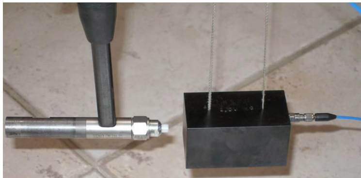
Figure 25 – The calibration mass used to verify the calibration/sensitivities of the hammer and accelerometer.
