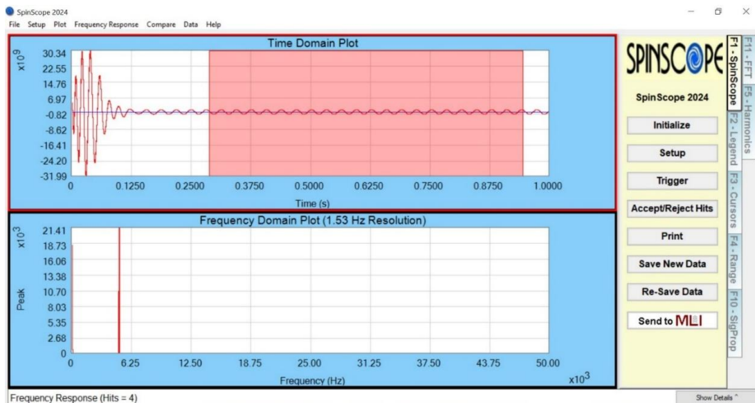
Figure 11 – Main SpinScope screen when using the Frequency Response Module, featuring an additional button in the side panel for accepting/rejecting hits.
