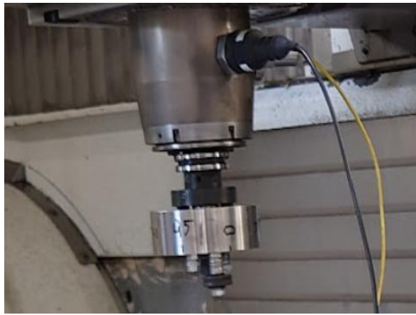
Figure 32 – Test configuration for evaluating the Balancing module with the DMU machining center.
