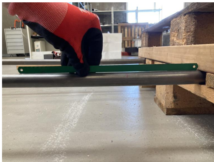
Figure 11: demonstration of the small deflection after bending.
