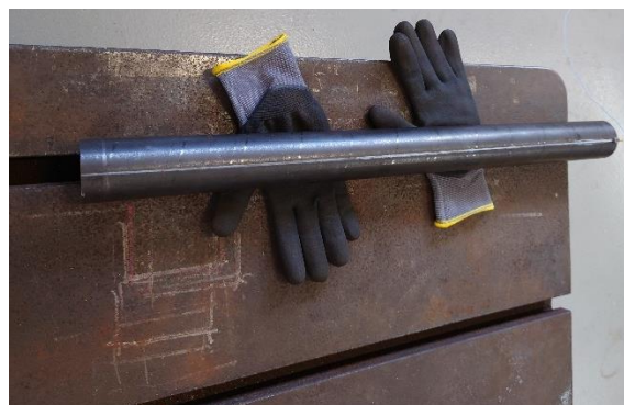
Figure 2: Placement of the test specimen during tap tests when removed from the experimental set-up.
