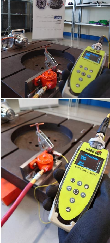
Figure 6: Pneumatic motor - Vibration analysis.
