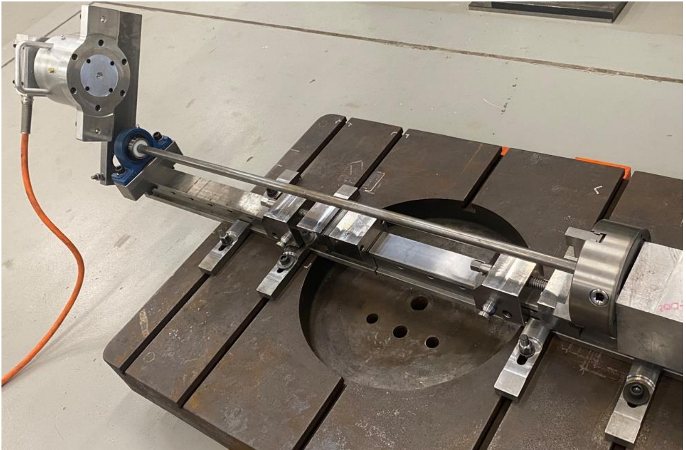
Figure 8, \varnothing 25 mm bar test set-up. Silver VSR vibrator mounted on torsional arm. Bar is fixed in one end and supported with a bearing in the other end. This set-up is used both for app. 3000 mm bar and app. 1500 mm bar. The vibrator is balanced vertically to eliminate static load and hereby also overload of the bar.
